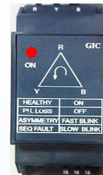
Power Scanner in ODU
